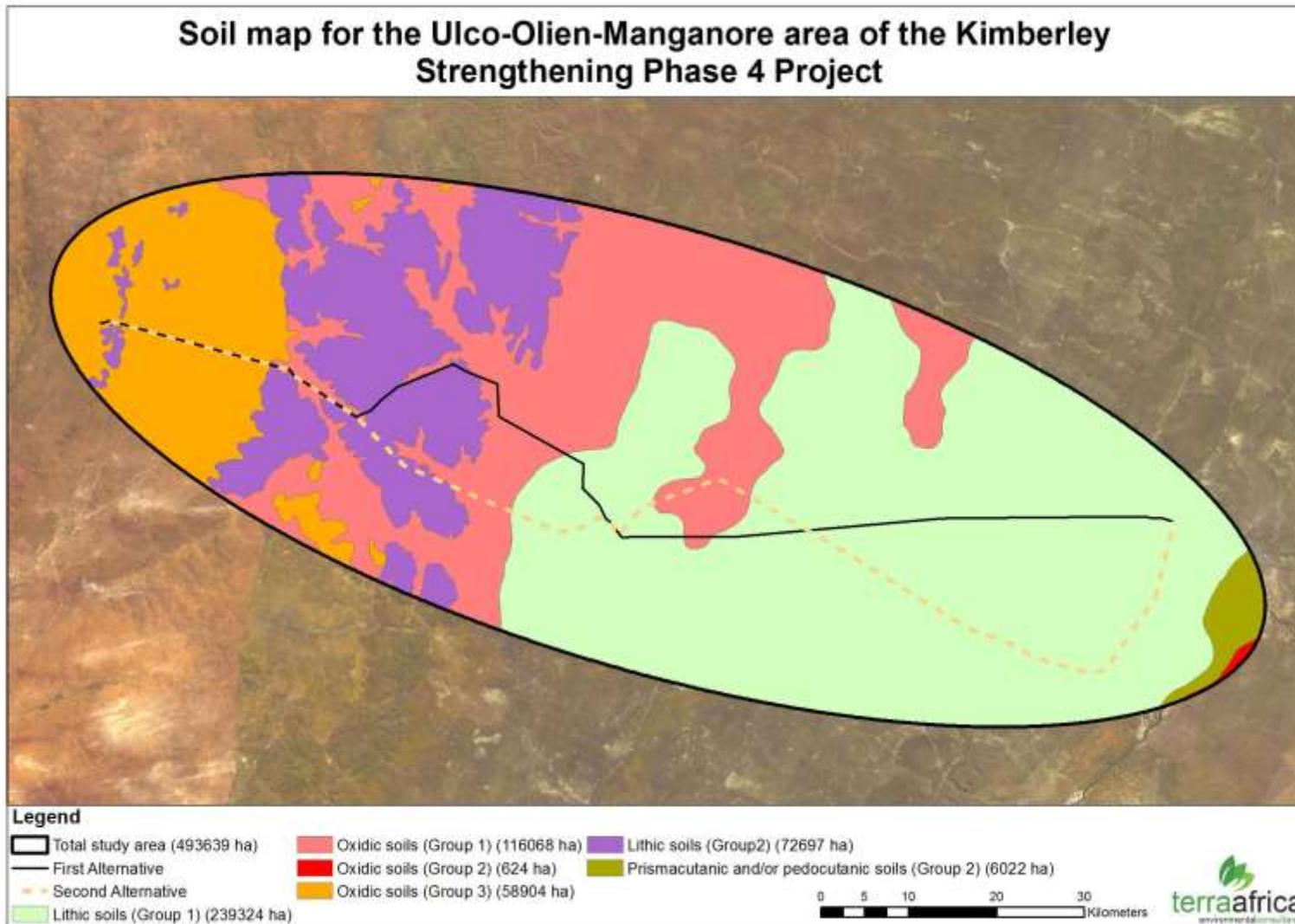
**Figure 26: Soil map for the Ulco-Olien-Manganore area of the Kimberley Strengthening Phase 4 Project**
